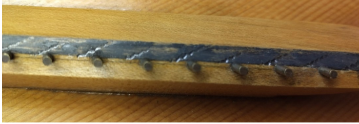
Figure 3: marks of open wound strings left on bridge.
