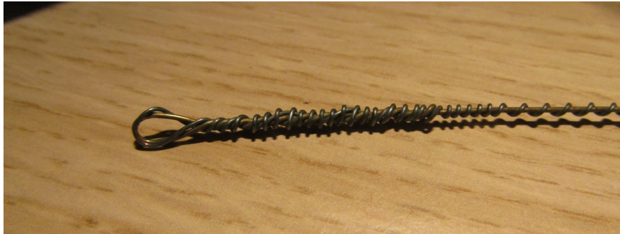
Figure 1: A typical open wound string of a square piano with the cover wire around the hitchpin loop.
